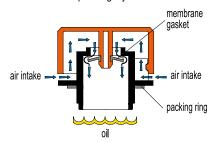
The membrane gasket warps and lets air inside the reservoir due to the effect of the vacuum which is created by the liquid discharge.
